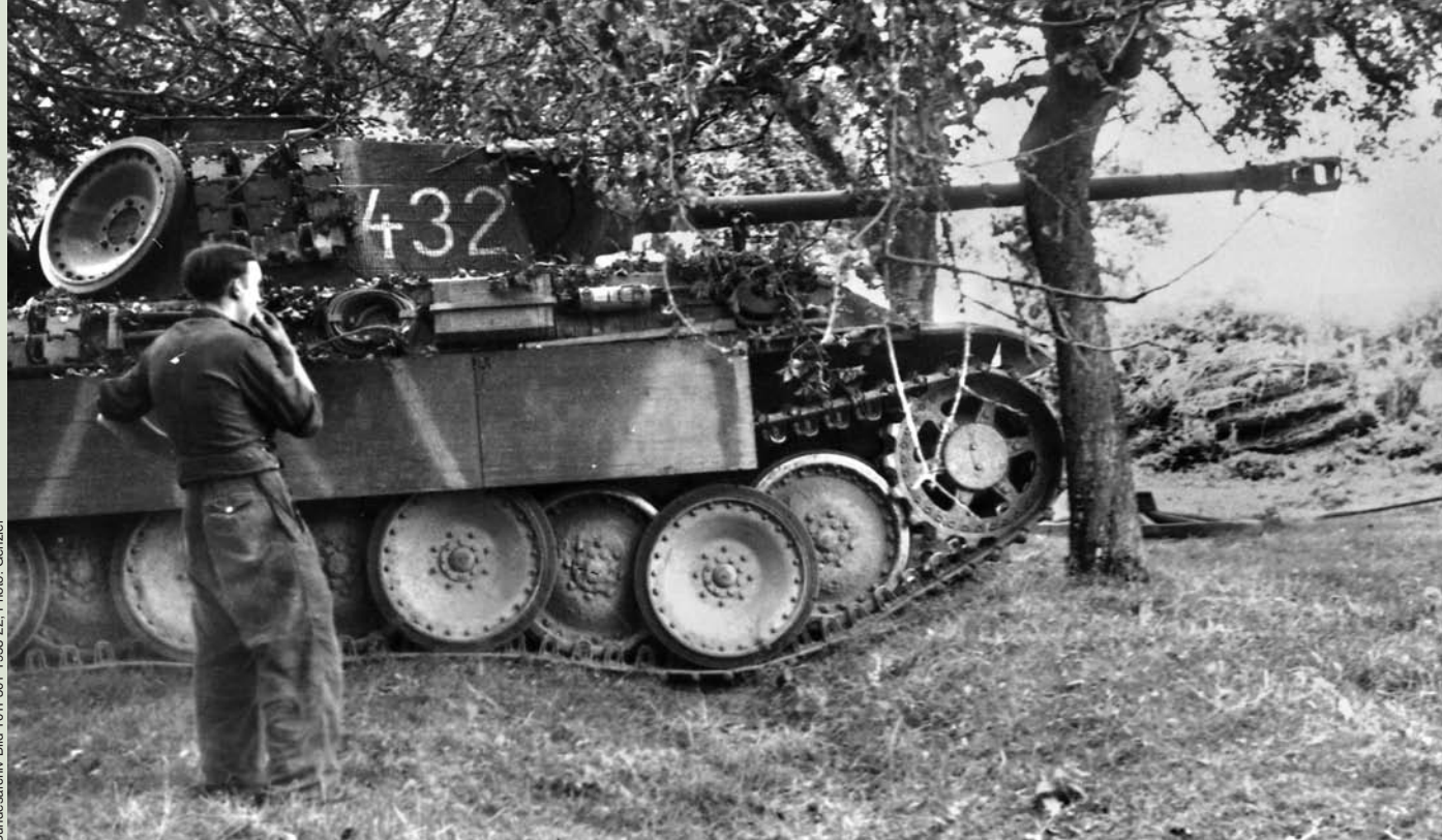
The German Panther outclassed the American Sherman tank in nearly every respect except speed. Introduced in 1943, the Panther boasted a high-velocity 75mm gun and its thick, sloped frontal armor stopped rounds from Shermans and M18 Hellcat tank destroyers.
